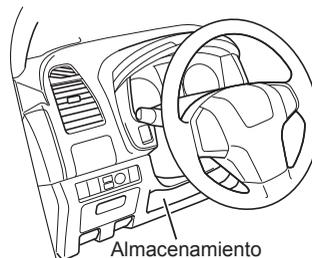
**Parte inferior central del panel de instrumentos**
