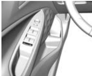
Pulse el interruptor
